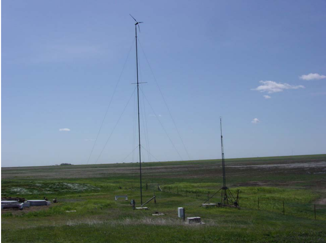
Fig. 1. Southwest Windpower H-80 mounted on a 19.2 m tilt-up guyed pipe tower (Bushland, TX).
