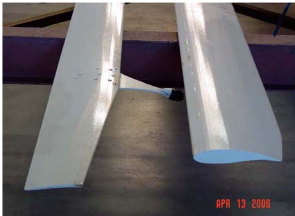
Fig. 11. Upper Surface (Suction Side) of Bergey 10 kW Blades Tested.
