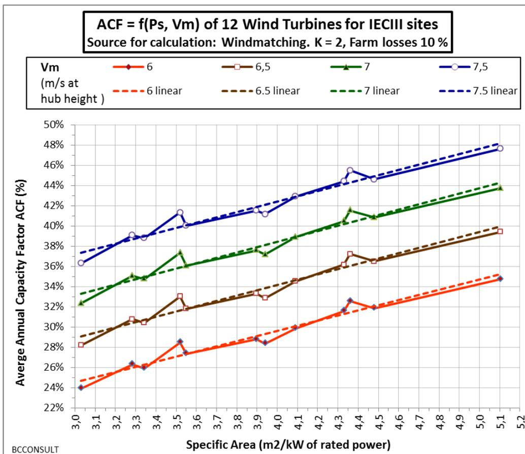
Figure 2: Average annual capacity factors (ACF, %) of 12 models of wind turbines for IECIII sites
