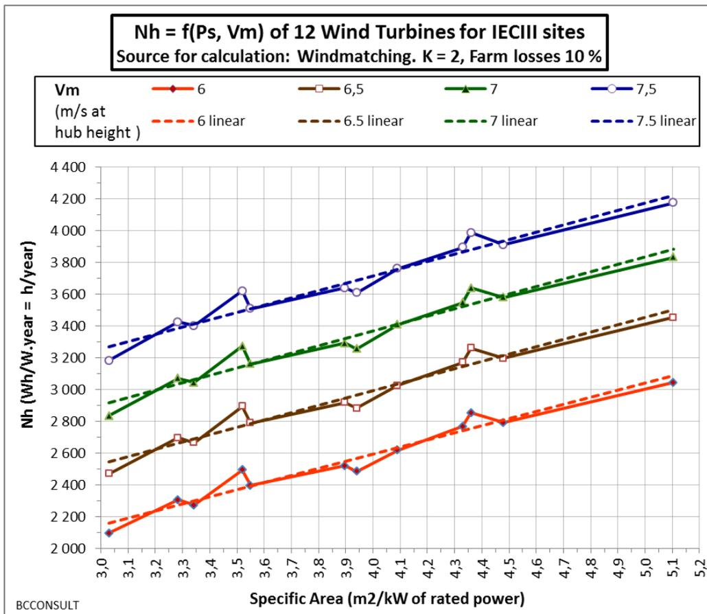
Figure 1: Yearly equivalent full load hours (Nh, hours/years) of 12 models of wind turbines for IECIII sites
