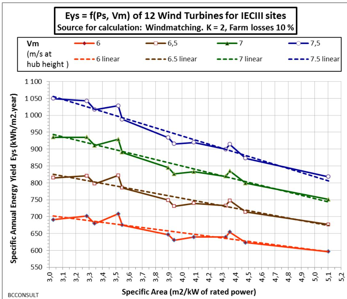
Figure 3: Specific Annual Energy Yield  $E_{ys}$  (kWh/m<sup>2</sup>.year) of 12 models of wind turbines for IECIII sites
