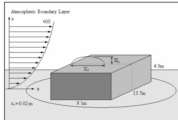
Figure 2: Building configuration with separation bubble defined.
