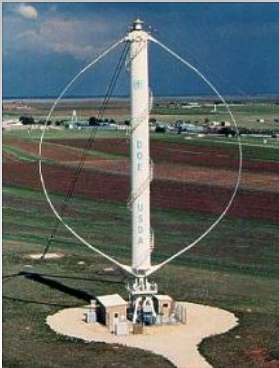
Sandia 34 m testbed Darrieus “eggbeater” Source: Sandia National Labs
