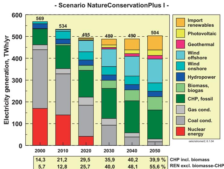
**Fig. 19: Power generation by power plant types and energy sources in the NatureConservationPlus I scenario. The increase from 2030 onwards is due to the provision of electricity for hydrogen production (2030 = 10 TWh/a, 2040 = 33.5 TWh/a and 2050 = 70 TWh/a).**
