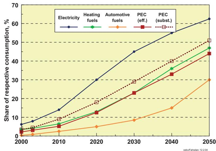
**Fig. 26: Growth of renewable energy sources in the extension scenarios, shown separately for individual supply sectors (share of final energy), and growth of primary energy input between 2000 and 2050 (with distinction between efficiency method and substitution method).**
