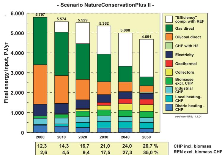
**Fig. 20: Structural changes in the heat market in the NatureConservationPlus II scenario as a result of building improvement and other efficiency measures and the extension of combined heat and power generation and of renewable energy systems by 2050.**
