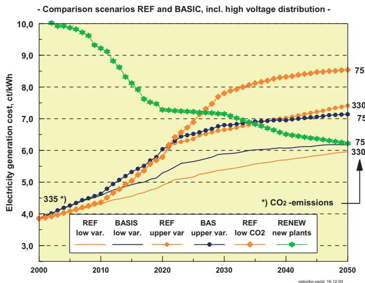
**Fig. 23: Comparison of average electricity production costs in German power supply sector (including high-voltage distribution) for different variants of energy price trends, and with a typical cost curve for new installations for utilization of renewables (low CO<sub>2</sub> = sequestration of CO<sub>2</sub> from fossil-fuel power plants from 2020)**
