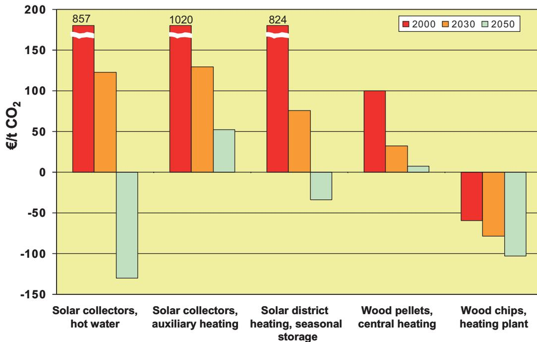
**Fig. 7: CO<sub>2</sub> avoidance costs of heat production from renewable energy sources. Based on: heat supply for a single-family house with a mix of gas-fired condensing boiler and oil-fired low-temperature burner in line with the reference scenario. Development of heating fuel prices: “middle variant”**
