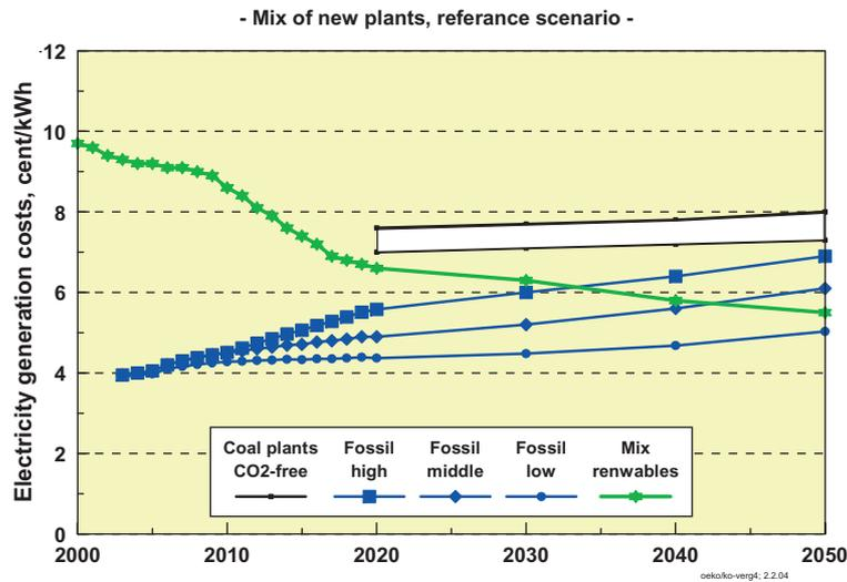
**Fig. 27: Electricity production costs of new fossil-fuel plants in the reference scenario for three price variants, and for coal-fired power stations with CO<sub>2</sub> retention (from 2020) and a representative mix of renewable energy systems (upper = middle + 15 €/t CO<sub>2</sub> mark-up)**
