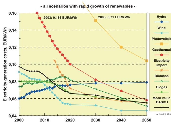
**Fig. 22: Representative cost curves of the individual mixes of reference technologies (technology groups; new installations from 2000 onward) for individual renewable energy systems, and cost curve of the mean of the entire mix in the scenario BASIC I, (interest rate 6%/a).**
