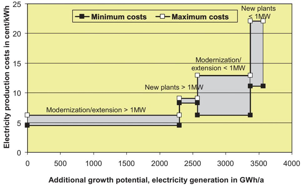
Fig. 5: Supply curves for additional hydro power potential in Germany.
