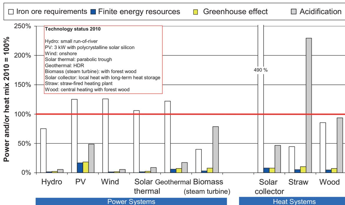
**Fig. 8: Results from Life Cycle Assessment of various renewable energy systems (sample selection of systems and environmental impacts). The representation is based on a future electricity mix in accordance with the reference scenario or a small consumer heat mix.**
