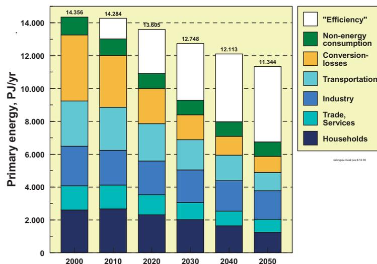
**Fig. 17: Trends in final energy demand and the resulting primary energy (efficiency method) in the extension scenarios. “Efficiency” is taken to mean the additional reduction compared with the reference scenario that can be achieved by means of increased efficiency measures and the increased extension of combined heat and power generation.**
