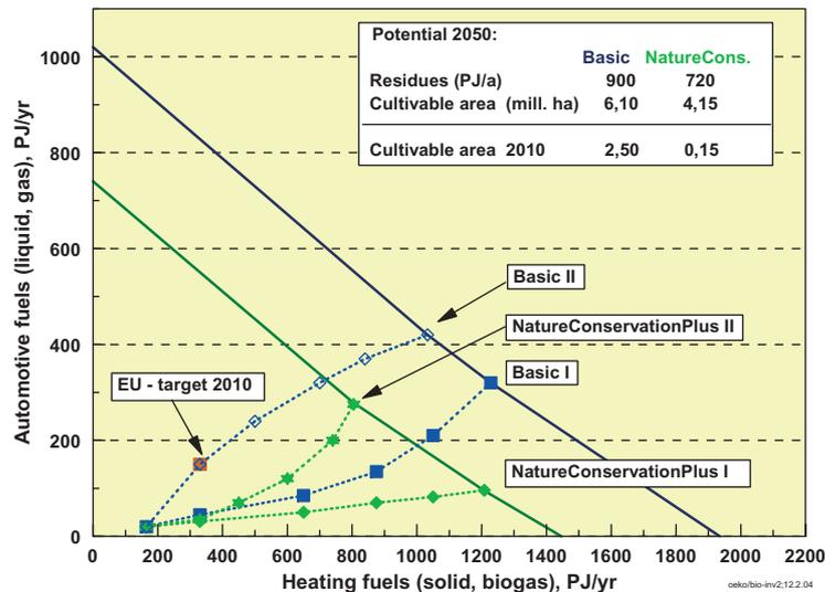
**Fig. 18: Two paths each for possible utilization of the biomass potentials determined for stationary and mobile utilization in the scenarios BASIC and NatureConservationPlus. Each mark corresponds to an interval of 10 years, starting in 2000.**
