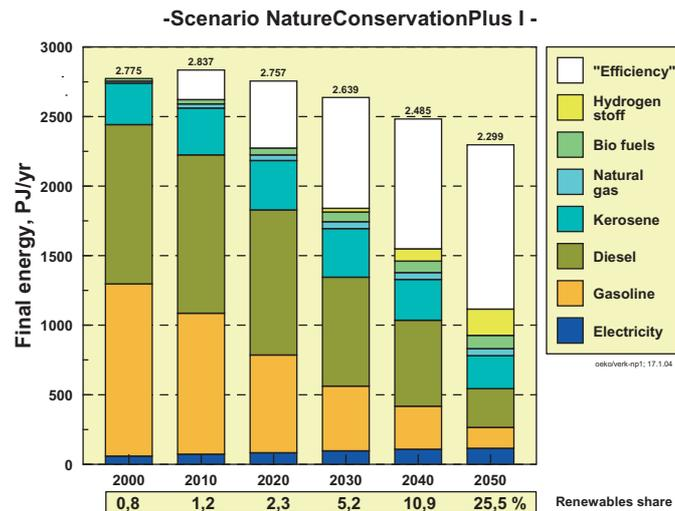
**Fig. 21: Structural changes in automotive fuel supply in the NatureConservationPlus I scenario, showing the relevant shares due to renewable energy sources up to 2050.**
