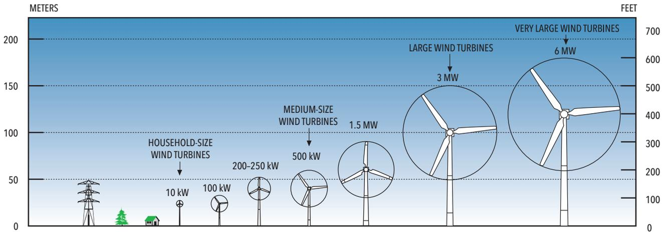
Figure 2-2. Relative size. Wind turbines today span the gamut from micro turbines only 1 meter (3.3 feet) in diameter to very large turbines with rotors greater than 100 meters (328 feet) in diameter. Very large wind turbines intercept 1,000 times more of the wind stream than micro turbines.
