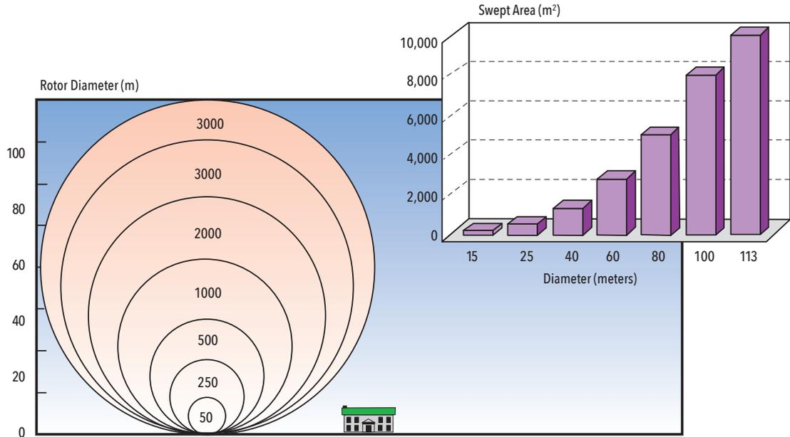
Figure 5-1. Medium-size and large wind turbines. The area swept by large wind turbines has increased steadily since the early 1980s. Today's wind turbines are 50 times larger than those of the early 1980s.
