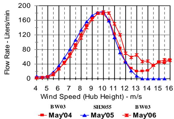
Fig. 13. Power Curves of Bergey 10 kW Blades at 75m head (Bushland, TX).
