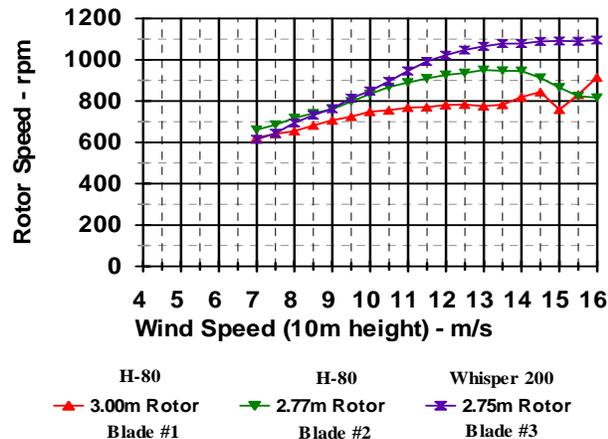
Fig. 9. Effect of Blades and Wind Turbine on Rotor Speed (75m head, Bushland, TX).
