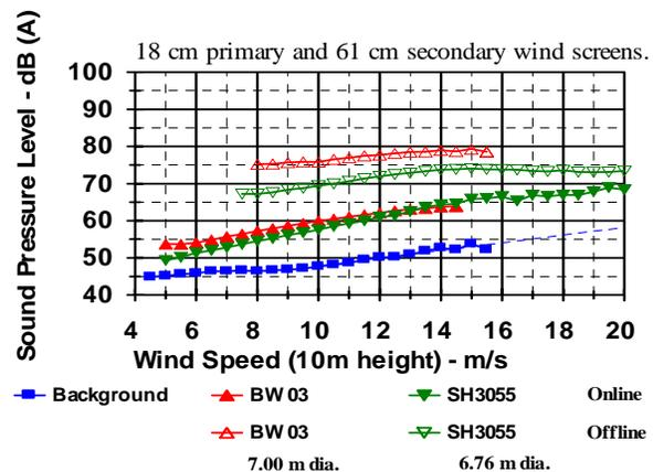
Fig. 17. SPL of Bergey 10 kW Testing (Primary & Secondary Windscreen).
