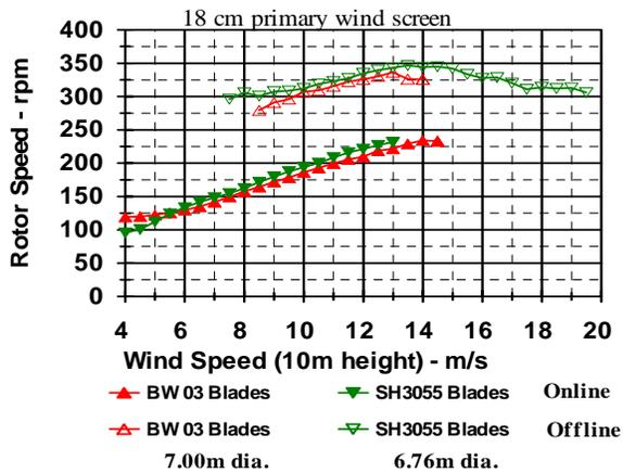
Fig. 18. Rotor Speed of Bergey 10 kW Testing (Only Primary Windscreen).
