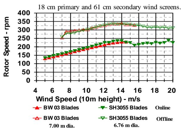
Fig. 16. Rotor Speed of Bergey 10 kW Testing (Primary & Secondary Windscreen).
