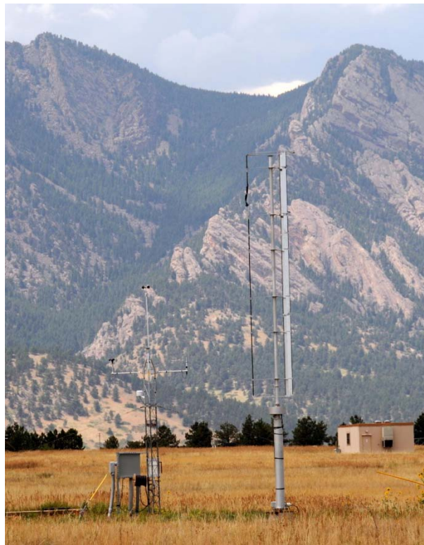
Mariah Power's 1.2-kW vertical-axis Windspire Giromill wind turbine installed for testing at the NWTC.
